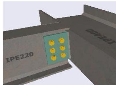
All connections can transfer **shear force in the major and/or minor axis** as well as **compressive or tensile axial force**. Each component is checked according to the final provisions of **EN 1993-1-1** and **EN 1993-1-8**, with the generalized 3D loading that includes forces in all 3 directions as well as bending moments due to load eccentricities.
