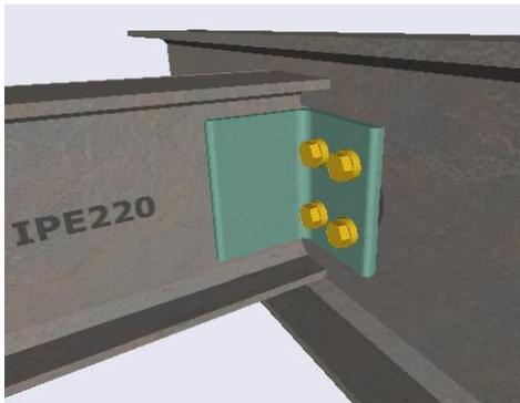
For the verification of the connections in tensile loading, **full T-stub analysis** is performed on the bolted assembly that includes the angle cleat(s) and the main member's flange or web.
